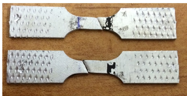
Fig. 2 fracture of sample after uniaxial tensile test
